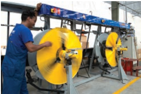
Manufacturing coils on the Buteline Pipewinder
